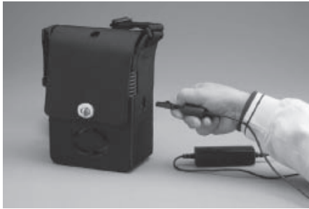
Figure 5: Internal Battery Charging
