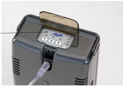
Figure 15: Indicator of Required Inspection/Service
